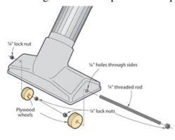
battled with to keep it from sucking the floor nozzle tightly to the shop floor. You solve the problem by cutting and mounting a set of small plywood wheels to the underside of the nozzle as shown. The wheels roll easily across the floor, even through
