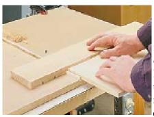
Next inset a strip of wood into the top to serve as an index pin for spacing the dadoes, see Figure 1. Make sure that the distance between the router bit and the index pin equaled the
