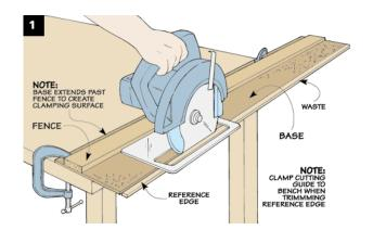
The nice thing about this cutting guide is it has a reference edge that aligns the saw blade with the layout line. By aligning this edge with the layout line, the blade makes a perfectly straight cut exactly where you want it.
