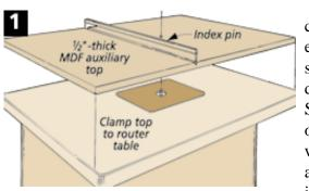
c u t t i n g e v e n l y spaced dadoes is easy. Simply butt one of the workpieces against the index pin and
