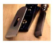
Chisels, Plane Blades and Carving Tools. Because the cutting edges of these tools often form acute angles (15 degrees to 30 degrees), they must possess a high degree of toughness. These tools must be able to hold an edge over long use, but the edge must
