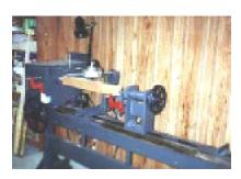
and skews. Each tool has a changable cutting tip made of HSS. The lathe itself has 14 speeds and a 20 inch swing. Gene is looking into a varible speed motor to replace the series of pulleys he fabri-
