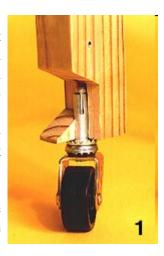
To install the socket for a stem-mount caster, drill a hole the size of the socket's outside diameter straight into the bottom of the leg. Drill about 1/4" deeper than the length of the caster stem. Drive the socket into the drilled hole, then snap the caster into it. Non-socketed stem-mount casters fit into a hole the same size as the stem diameter.
