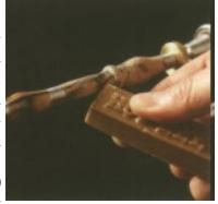
speed that's safe for the size of your workpiece). Then, starting at one end of the turning, press the stick of finish against the surface, as shown in the photo at left. Move it slowly toward the other end, covering the surface evenly. Apply the stick to the lower portion of the turning, where it's rotating away from you.
