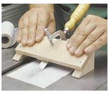
The problem is holding the chisel at a consistent angle as you sharpen. To do this, you clamp the chisel to a simple sharpening guide (see photo).
