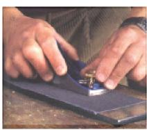
A. Flatten the sole: Flattening the sole of a plane is tedious, but the payoff is a smooth and accurate response to the blade and mouth adjustments.
