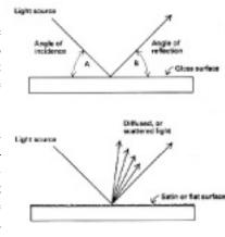
makes a reflected image less distinct because less light reaches your eye. Generally, the finer and more uniform the scratch pattern from polishing, the glossier the sheen. From *Fine Woodworking*.
