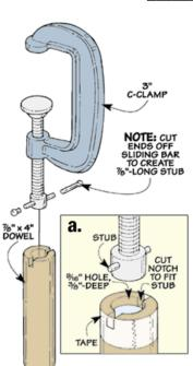
Sometimes the sliding bar on a C-clamp, used to tighten the clamp, gets in the way. Before each turn, you have to slide the bar all the way to the opposite side. It's a pain.
