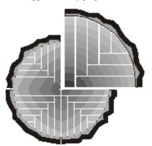
ing). In contrast, plain sawn lumber has the growth rings parallel to the board's broad face. Quarter sawing produces both Quartered and Rift lumber.
