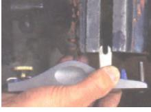
front edge of the plane is smooth and free from nicks or burrs that could mar the workpiece.
