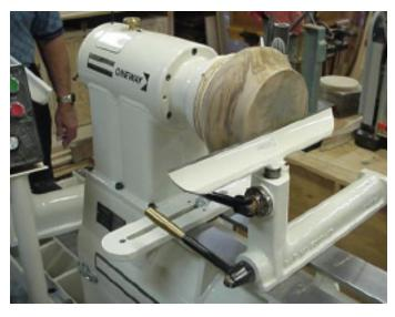
The lathe has a swing over the bed of 20" and a maximum headstock to tailstock distance of 36". The bed can be extended to 5 feet. Outboard of the headstock, it can handle up to 44" stock (though you'll need a helping hand to lift that big log up there).
