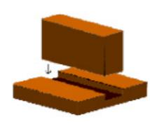
not too wide, otherwise the joint will not be tight enough to work. It is far better to start with too tight a groove and widen it. A router is not always the best tool to use however. If the groove is to hold a piece of 1/4 inch (or smaller) plywood, you should use a circular saw in-
