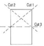
though it is tempting to cut straight down into the tenon, a safer way is to cut at a 45 degree angle, as shown in the diagram, before finally cutting in a horizontal manner. Doing this reduces the risk of cutting into the tenon on the side furthest away from you (see diagram above).
