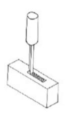
end. Once you have done the entire length of the mortise, scrape out the loosened waste wood. Then begin again, cutting down another 1/4" and so on. Once you are down to just over half-way down into the joint, turn the wood over and start in from the other side. Once the hole is made, clean up both ends, cutting back that extra 1/8".
