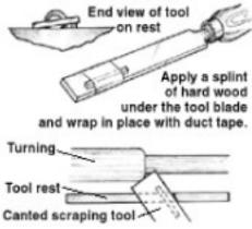
Not all so-called "scrapers" are beginnes. Pat-ternmakers invariably scrape to the finished shape because this method offers more control and a mechanical shape that is exactly "to the drawing".
