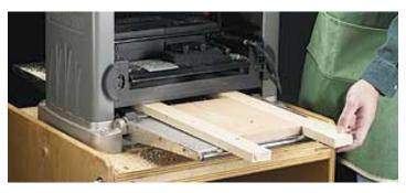
ommended. It can get caught between the infeed and outfeed rollers, causing it to lift off the planer bed. At best, this causes severe snipe (a deeper cut near the end of a board.) At worst, the board can get chewed up, damaging the cutterhead in the process.
