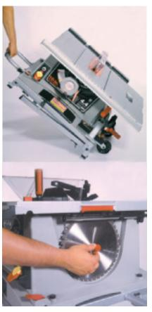
depth of cut is 3 1/8" at  $90^{\circ}$  and 2 1/4" at  $45^{\circ}$ .
