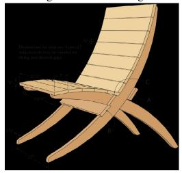
You will have to tape several pieces of paper together to get the full-size image and may find some minor discontinuities – flat spots and abrupt changes in curvature. Rather than build these into the chair, use a flexible batten, spring it into the right shape and redraw the curves with a felt-tipped pen. Continues next page.
