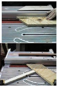
the fence. Position the featherboard firmly against it and clamp to the table. The feather board should be placed firm enough to keep the stock against the fence but should not make it difficult to push the stock into the cutter. A small scrap can be clamped against the featherboard as seen in the picture to the right. This will help keep the featherboard from slipping as you cut. For preventing blow-out at the end of the stock, clamp a peice of scrap at the end. From Woodzone.com
