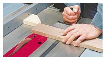
provides clearance between the rip fence and the saw blade so the cut-off pieces don't get trapped (and kick back).
