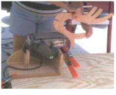
ordinary belt sander into an expensive Grizzly combo belt/disc benchtop sander. With this jig and my old Sears Craftsman belt sander, I can finish inside curves, flatten stock and I even use it to sharpen my lathe gouges and scrapers. *Barry Humphus*.
