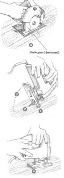
rial, you lower the base plate flat against the surface. At that point, push the saw forward through to the end of your cut. *Barry Humphus*.
