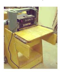
bench. The bench securely holds the planer while in operation while providing plenty of support for feeding long work peices. The support table folds up for storage and the lower part of the bench has a large storage drawer for tools. Not having a surface planer of my own, I've used George's several times
