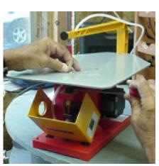
place in the shop. It has the same 1700 RPM induction motor as their larger saws (but without built-in varible speed). Because it is an induction motor, you could add an after-market varible foot switch. The table is 11" x 17" in size. While it does not need to be bolted
