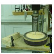
ShopNotes. The unit is driven by his drill press, is adjustable for various blades (including turning tools) and works especially well on chisels and plane irons. It consists of a two-inch thick disk wrapped with abrasive paper or cloth. He covered the top
