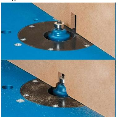
Many times, adding an auxiliary fence is enough. But you can also create a smooth, seamless tabletop and eliminate any gaps here as well. After positioning the fence, you clamp a larger piece of hardboard to the tabletop tight against the fence.
