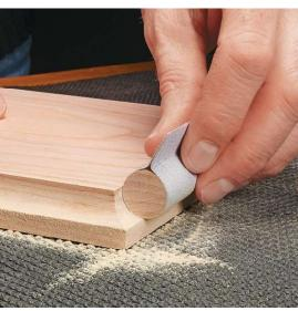
You can flex the long thin blade to get right where you need to sand. Simply wrap the adhesive backed paper around the knife and go after that tight space.
