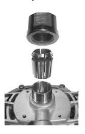
Picture a collet at work. As you tighten the collet nut, you drive the increasing taper of the collet cone into the matching decreasing taper milled into the end of the motor spindle. This squeezes the collet against the router bit shank, creating so much friction that the bit is locked in place and can't twist or pull out during operation.
