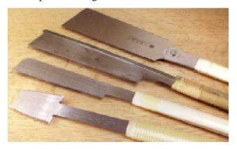
crimping the blade. This means the blades can be thinner, which results in a thinner kerf. The metal used for Japanese saws is harder and the teeth are tempered to a high degree. This keeps them sharper longer, but makes them almost impossible to resharpen. This isn't a negative, since the tooth geometry is complex, and with many of these you can replace the blade when it dulls.
