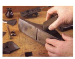
When all the parts are clean, free from rust, and sharp (if applicable), put the tool back together. As you do this, add a drop or two of light machine oil (automatic transmission fluid is light, acid free, cheap and makes a great general purpose light lubricant) to linkages
