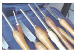
As the tool edges got worn with turning, Bill went next to his method of sharpening. He uses a 'slow' bench grinder (1,750 r.p.m.) with the white grinding wheels. Before sharpening, he'll clean and true the
