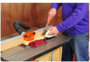
table should be fitted with a guard that covers the area immediately above the bit. Whenever possible, use a push stick or push block to propel the work
