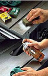
After removing any rust, seal the top by spraying on a protective topcoat, see bottom photo. Spray-on topcoat products are available at hardware stores and woodworking stores (Spray-on wax also works very well and is cheaper—from John Perry). In addition to rust protection, they also act as a sort of lubricant so workpieces slide smoothly across the table. From Woodsmith.
