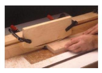
make sure the workpiece is pressed firmly against the router table top.
