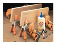
When edge-gluing several boards to make a panel, start by laying the boards in order on the pipe clamps to be certain that they're arranged the way you want them. Then, very carefully stand each board up on edge to apply the glue.
