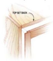
normal face frame is very obtrusive when viewed from the side. The solution is to attach rabbeted edging, as shown. This gives a finished look and the corner can sustain minor damage without marring the veneer. With a little easing of the corner, the face frame joint is almost invisible. You do have to cut the top and dividers so they are set back from the sides by the depth of the rabbet. From American Woodworker.
