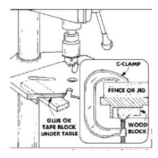
To solve this problem, cut and glue some scrap blocks to fit between the ribs. Because you may occasionally use the slots in the table, Iyou don't have to permanently fix the blocks to the table. So just put a few drops of glue from a hot glue gun on each scrap. Then stick the blocks between the ribs. (You could also use double-sided carpet tape to mount the blocks.)
