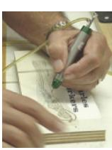
the turn of a lever. The system also features a water capture to keep the unit free of moisture from the compressor. The unit will run on about 40 psi from your shop compressor or from a tank of CO2 gas for very quiet operation. The down side is that it sounds just what it looks like: a denists drill. For some, that was a sound they'd like to forget.
