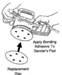
to cure to the rubber pad on the sander. After the adhesive cures, trim off any excess hook and loop pad (needed on the Dewalt and other smaller sanders).
