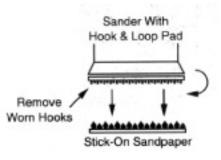
After sanding down to the rubber pad, apply a thin layer of the included adhesive to the rubber
