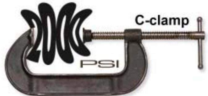
For example, the sliding bar clamp can produce about 400 psi – about twice what is needed for hard woods. The common pipe clamps gets up to 1,000 psi – some four times the needed pressure, while our old friend, the "C" clamp can put down a ton or more pressure at 2,000 psi. With a "C" clamp, you can make the wood say Uncle pretty quickly, squeeze out all of the glue and ultimately have a joint that fails.
