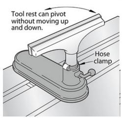
it's easy to lose track of the original elevation. Finding that exact spot again can try your patience. Slip a hose clamp from the hardware store onto the shaft of the tool rest in the position you want to return to and tighten it down as show. Then, go ahead and
