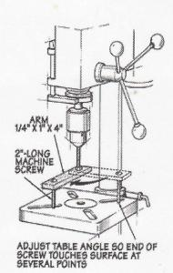
The jig takes about five minutes to put together. It's just a narrow piece of 1/4"-thick scrap wood that you cut about four inches long. Drill a hole through the face near each end and pushed a 2"-long machine screw through each hole, pointing in opposite directions. Nuts hold the screws snug so they are roughly parallel.
