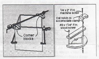
When gluing up the ends of rectangular projects, placing a bar or pipe clamp across opposite corners assures everything will be square after the glue sets-providing you keep the clamp from sliding off the corners. It was a problem I had when making the legs of the pool table I built last Summer. Besides, metal clamp jaws can easily mar or dent the workpiece.
