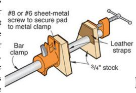
sheet-metal screws where indicated and attach the pads to the clamp jaws. For further protection, glue a leather facing to the clamping area on the pad. The pad design shown offers a bonus, too: The wide bottom allows you to stand the clamps on a bench or sawhorses for easier clamping.
