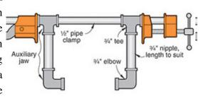
such jaws. Remove the sliding jaw of the pipe clamp and slip the tee fittings over the pipe with the open ends of the elbows facing inward. Replace the sliding jaw and clamp your project, protecting the wood from the rough iron of the elbow.
